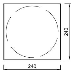
Openable cover with thermal insulation
