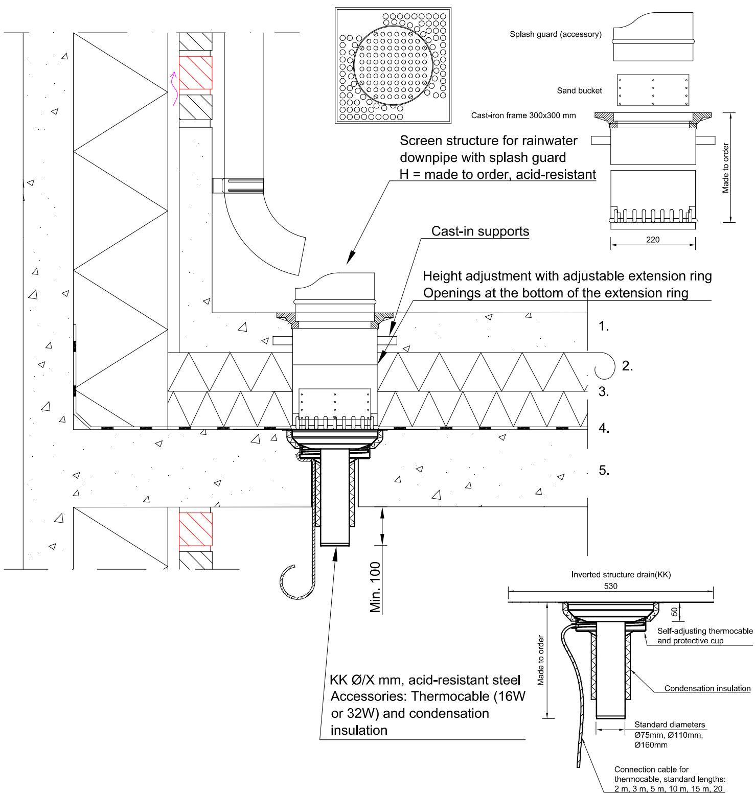
1. Reinforced concrete slab according to structural plan.
