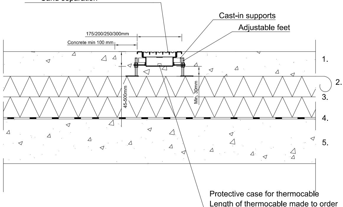
1. Reinforced concrete slab according to structural plan.
