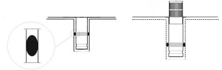
6. Following the installation of the renovation roof drain, the roofing contractor will ensure that the waterproofing is connected to the flange of the renovation roof drain.
